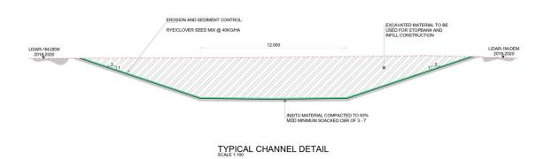
Figure 6-1: Typical detail for proposed channel cross-section.
