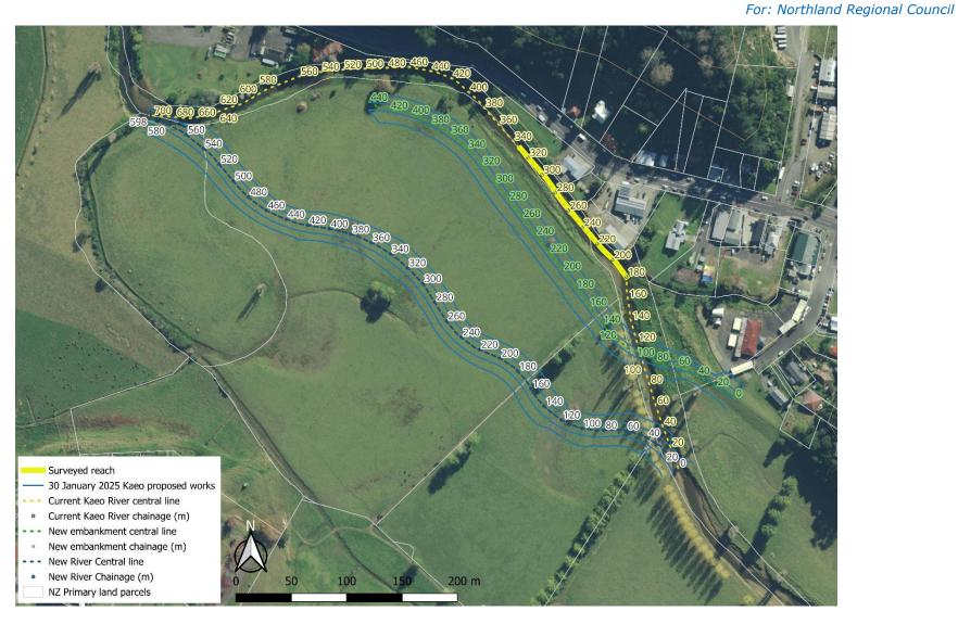
Figure 5-1: Proposed works to divert the Kāeo River and construct a floodwall (embankment).
