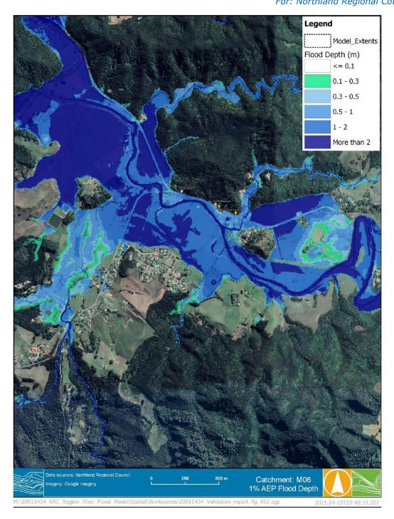
Figure 1-1: Model of water depth as Kāeo township during 1% AEP flood.
