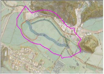
Figure1: Kaeo Phase 2 Flood Mitigation Project works area and 100m buffer marked in pink
