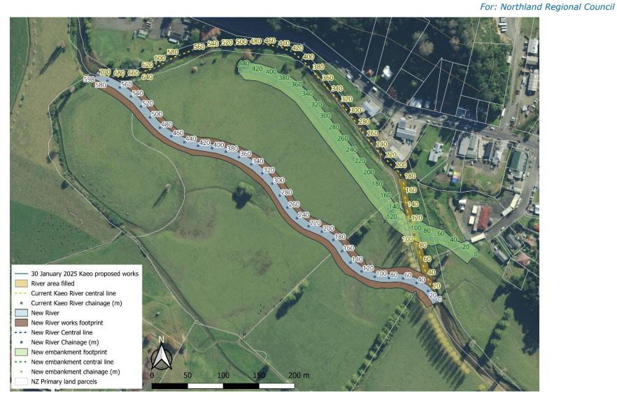
Figure 5-2: Areas of proposed works to divert the Kāeo River and construct a floodwall (embankment).
