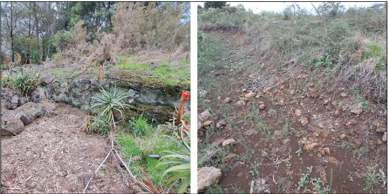
Figure 5: Juxtaposition of rock exposures within 5-10m of DBP in proposed Lot 1 (right - weathered volcanic cobbles and boulders) and proposed Lot 4 (left – massive basalt rock).
