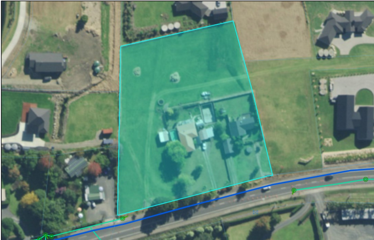
Figure 2: Snip from FNDC Water Services Map showing parent lot boundary (cyan), public stormwater (green) & public potable water (blue)
