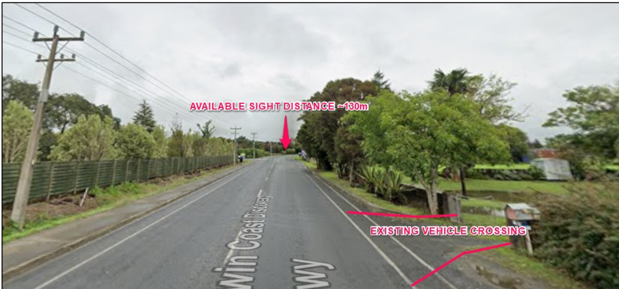
Figure 9: Annotated photo showing available sight distance from Vehicle Crossing 2 to the southwest
