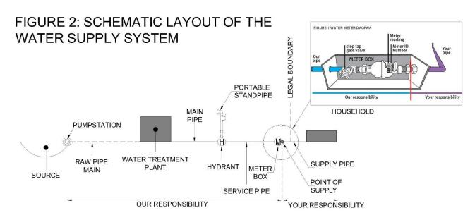
Part 2: Point of supply layout Illustration of typical layout of the fittings at the **point of supply.**
