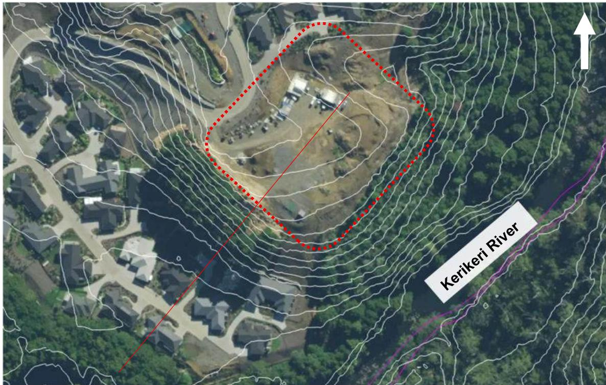
*Figure O: Aerial of subject Zone D development site and the surrounding slopes (Source: 2024 LINZ Basemaps Imagery, Northland LiDAR - pre-development 2.0m, contours, using QGIS). Development area in red dashed lines*
