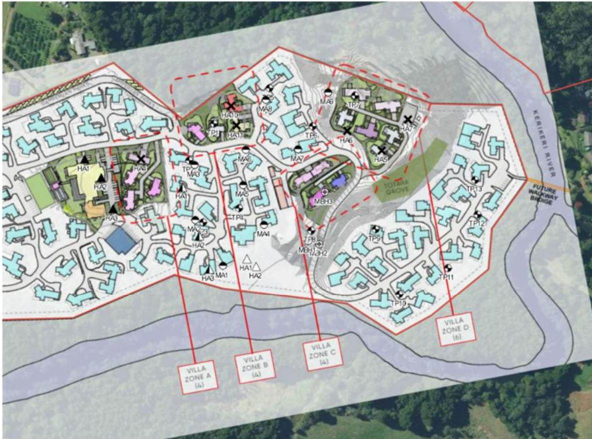
*Figure E: HGEA subsoil investigation plan with Foley Group Master Plan overlay*
