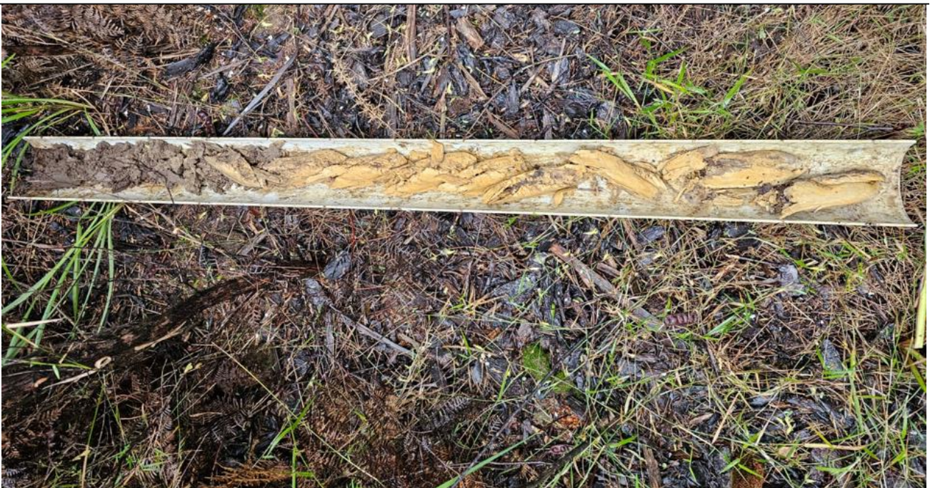
300mm topsoil over silty clay loam Class 5, (as per AC TP-58, Table 5.1)
