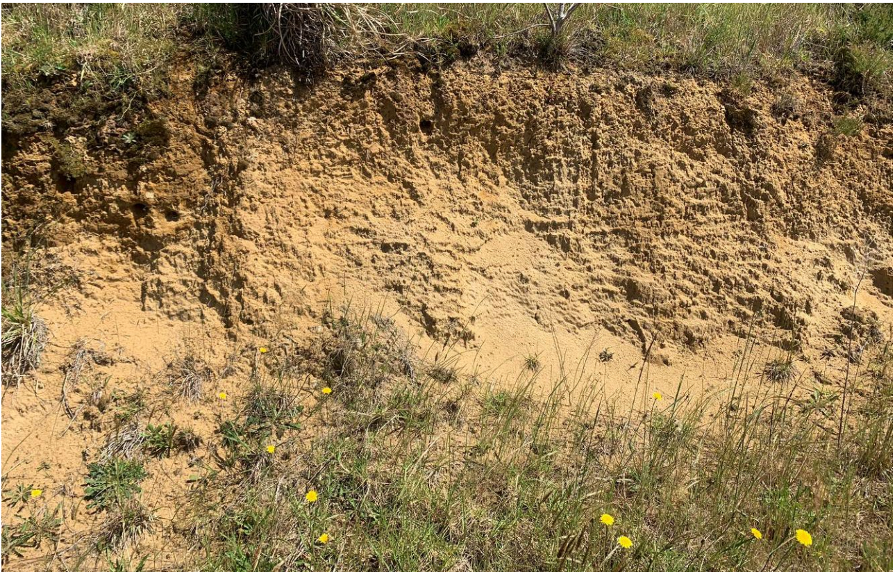
Photograph 2: Cut face showing soil type as category 3, orange, sand with good drainage.
