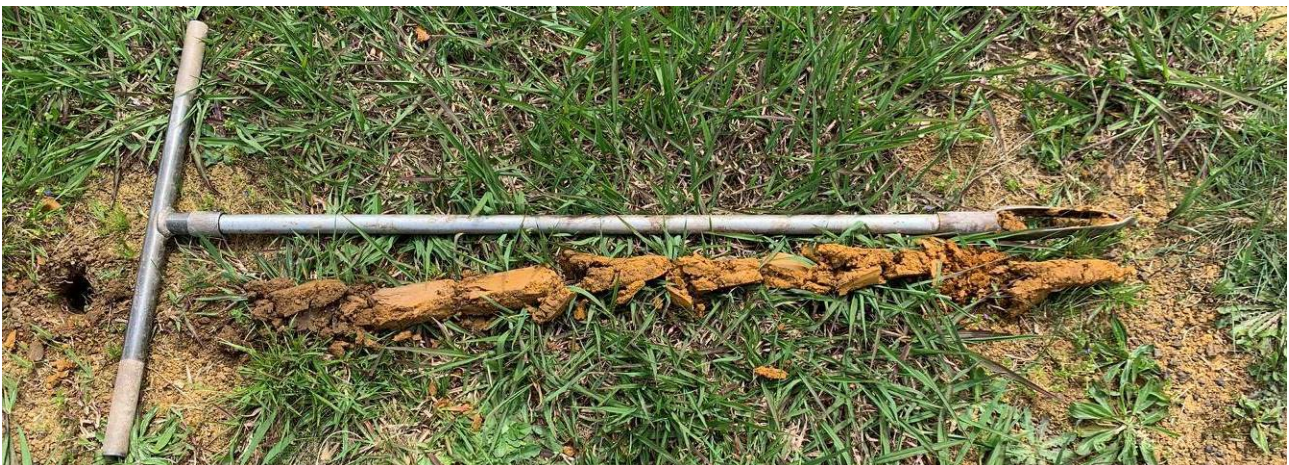
Photograph 2: Borehole showing no topsoil followed by category 6, slightly moist, brownish orange, slightly moist clay.
