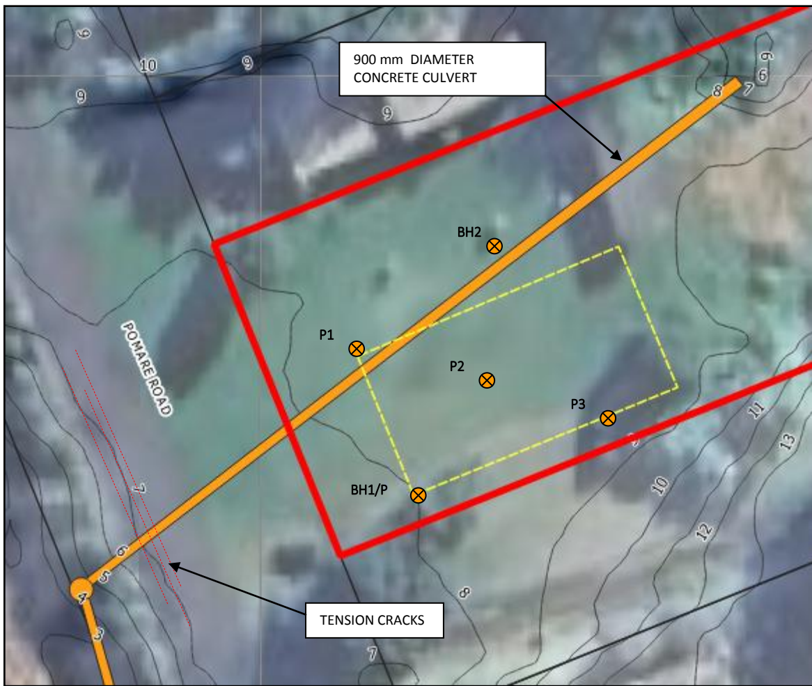
Figure 5. Geotechnical Test Location Plan
