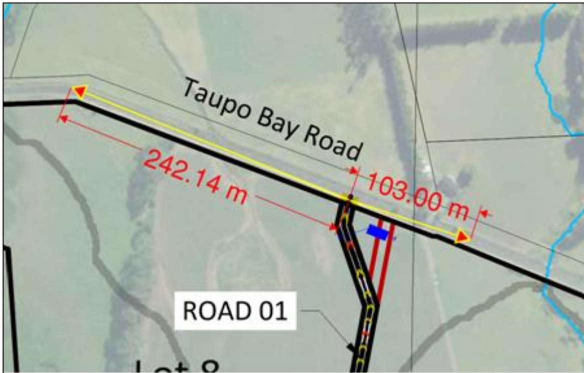
Figure 5: Road 1 Vehicle Crossing Sight Distances
