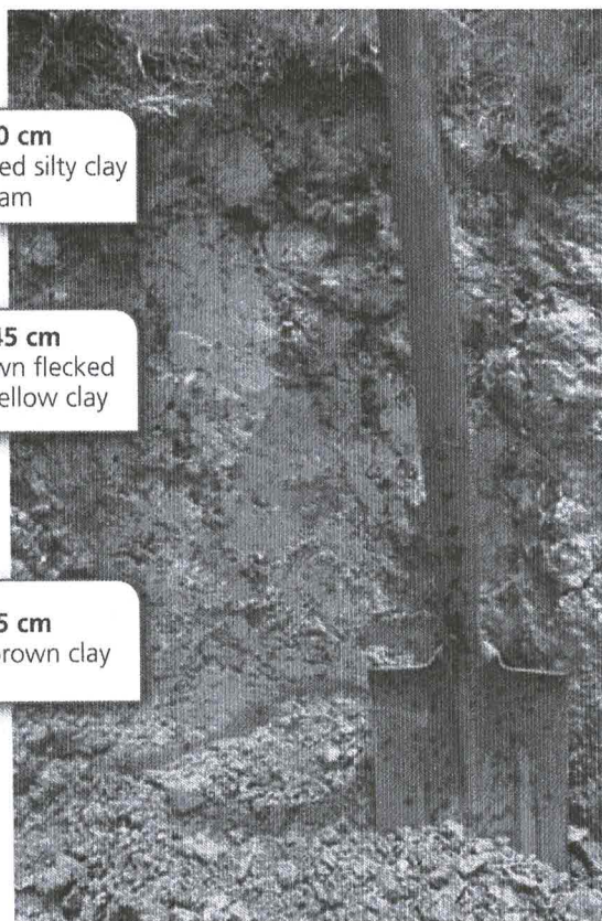
Rangiora clay, clay loam & silty clay loam (RA, RAH) soil profile
