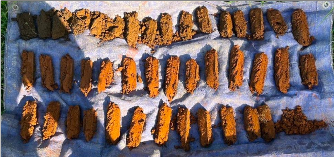
Figure 5: Site photograph of the typical HA soil arisings (HA01: 0.0m to 2.4m BEGL).
