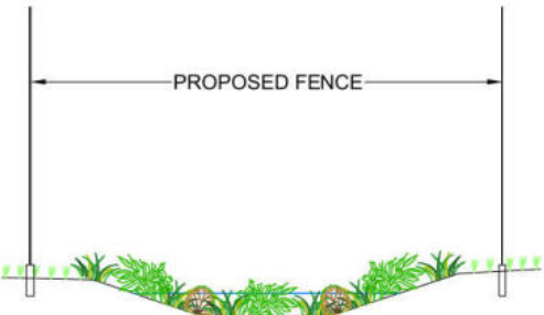
PROPOSED VEGETATED SWALE TYPICAL SECTION
