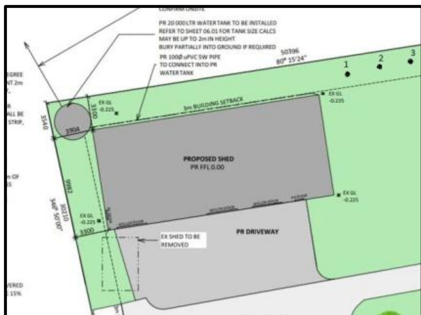
Figure 1: Approved Plan under RC 2300378 showing 20,000L tank which captures shed roof runoff, with overflow being directed to the adjoining site.
