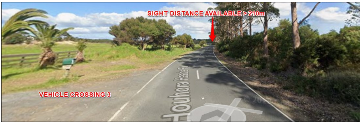
Figure 9: Annotated photo showing available sight distance from Vehicle Crossing 3 to the southwest
