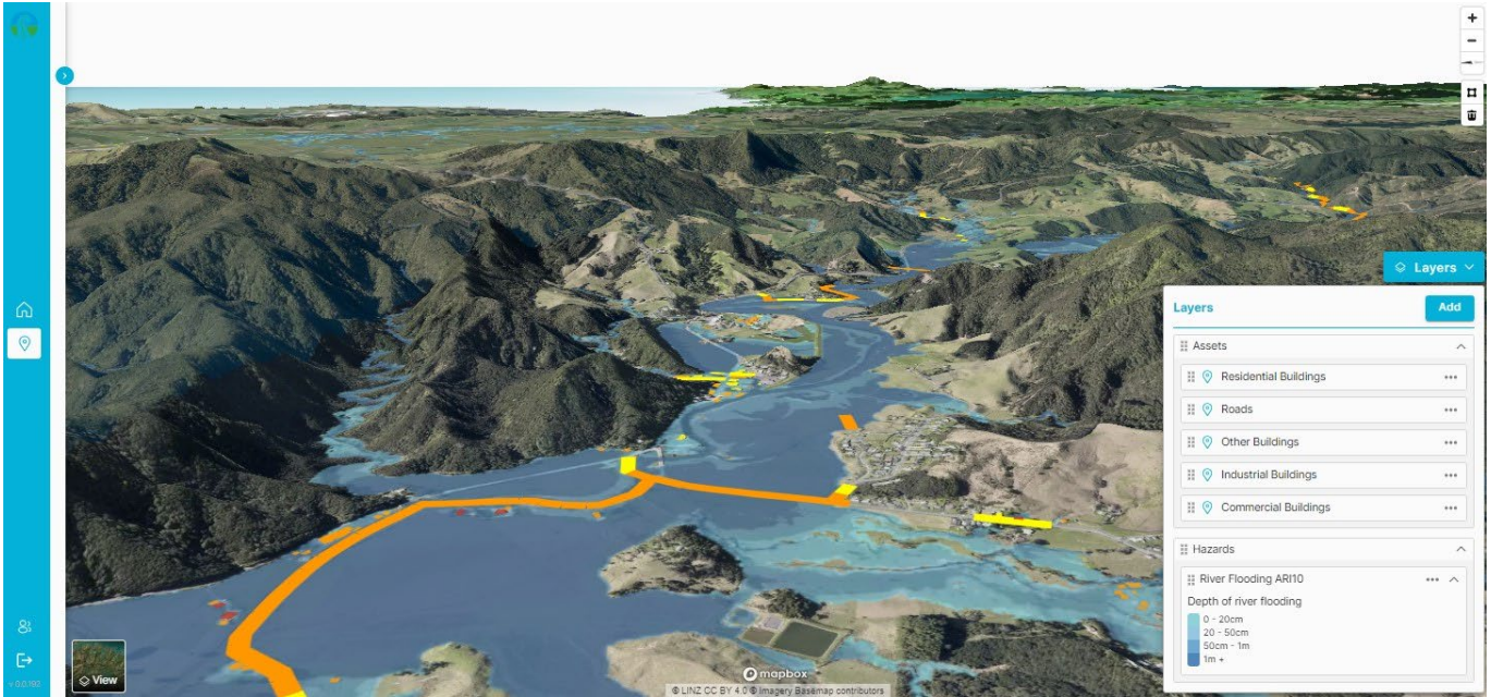
Figure 1. Risk assessment results as shown in the Resilience Explorer. Location near Kaeo, River flooding AR110
