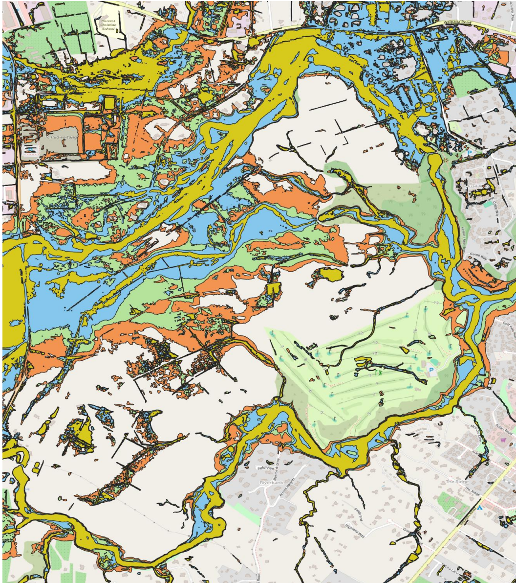
Figure E. New flood model extents for the KFO site. Orange = 2 x 1-in-100-yr; Green = 1-in-100-yr with climate change; Blue = 1-in-100-yr; Yellow = 1-in-10-yr flood events. Source Water Technology 2025.
