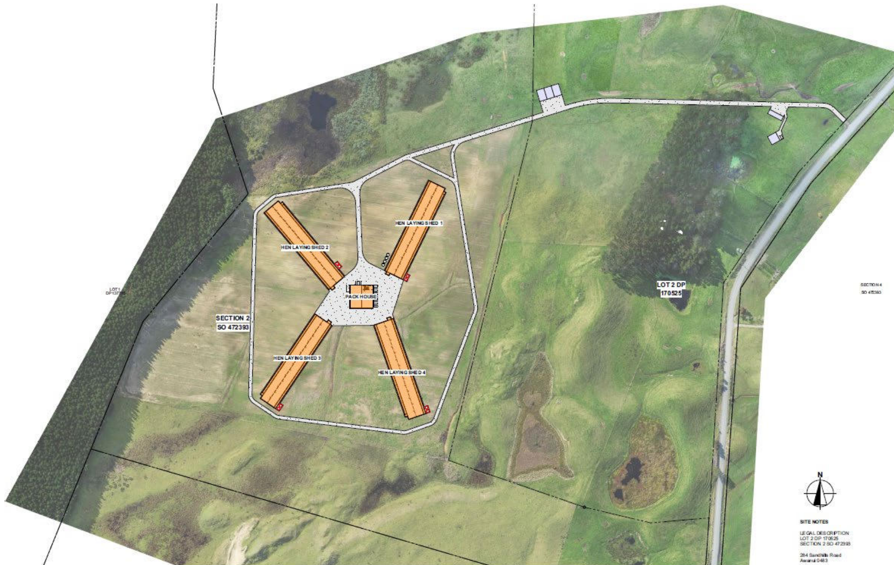
Figure 2. Site context plan showing proposed layout for free range chicken farm, four laying sheds and packhouse and associated accessways and structures (reproduced from Neo Architecture Studio Limited. Scale = 1:1500.
