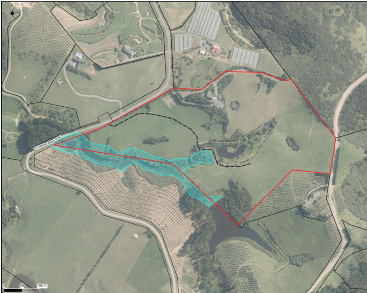
Figure 13: Indicative dam breach inundation map. Indicative inundation zone shown in blue shading.
