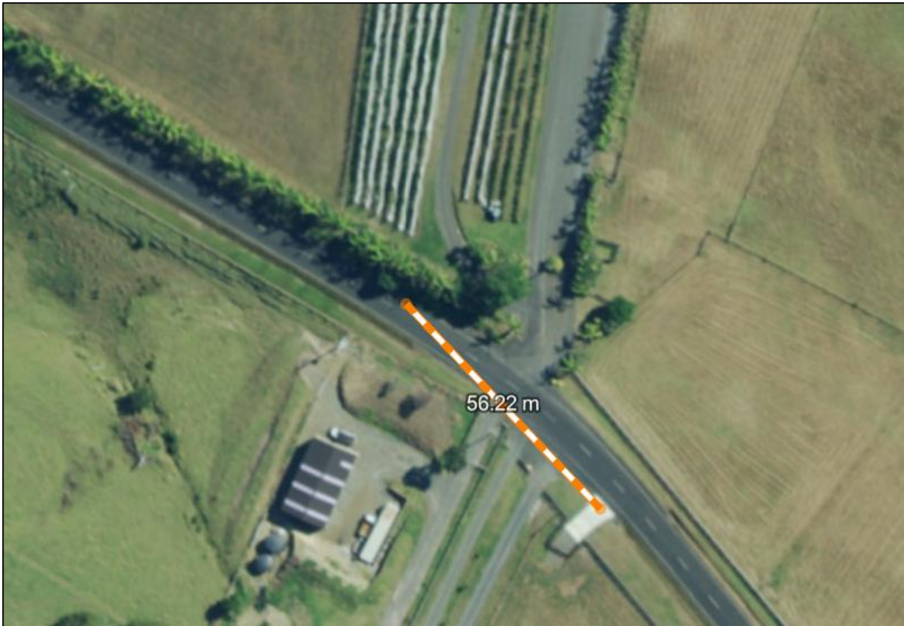
Figure 9: Aerial view of the existing Lot 1 vehicle crossing and annotated sight distance along Okahu Road southeast-bound lane from Lot 1 vehicle crossing (FNDC Atlas Maps).
