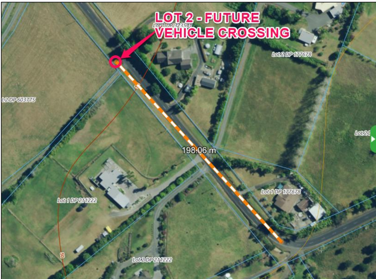
Figure 15: Aerial view of the site frontage and annotated sight distance along Okahu Road northwest-bound lane from Lot 2 vehicle crossing (FNDC Atlas Maps).
