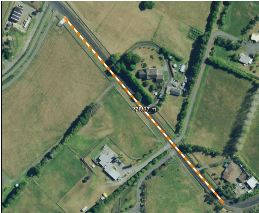
Figure 11: Aerial view of the existing Lot 1 vehicle crossing and annotated sight distance along Okahu Road northwest-bound lane from Lot 1 vehicle crossing (FNDC Atlas Maps).
