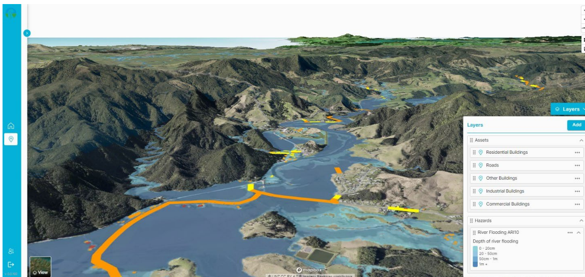
Figure 2. Risk assessment results as shown in the Resilience Explorer. Location near Kaeo, River flooding ARI10
