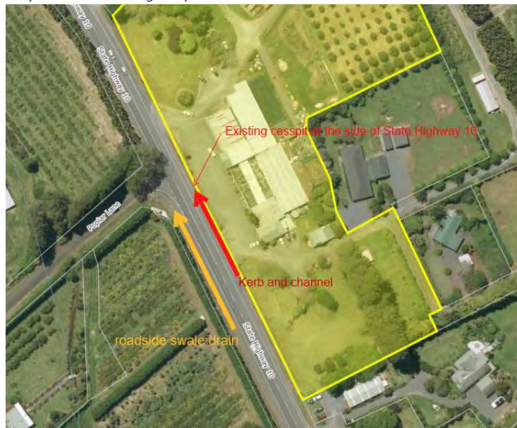
Figure 2: Stormwater system at State Highway 10
