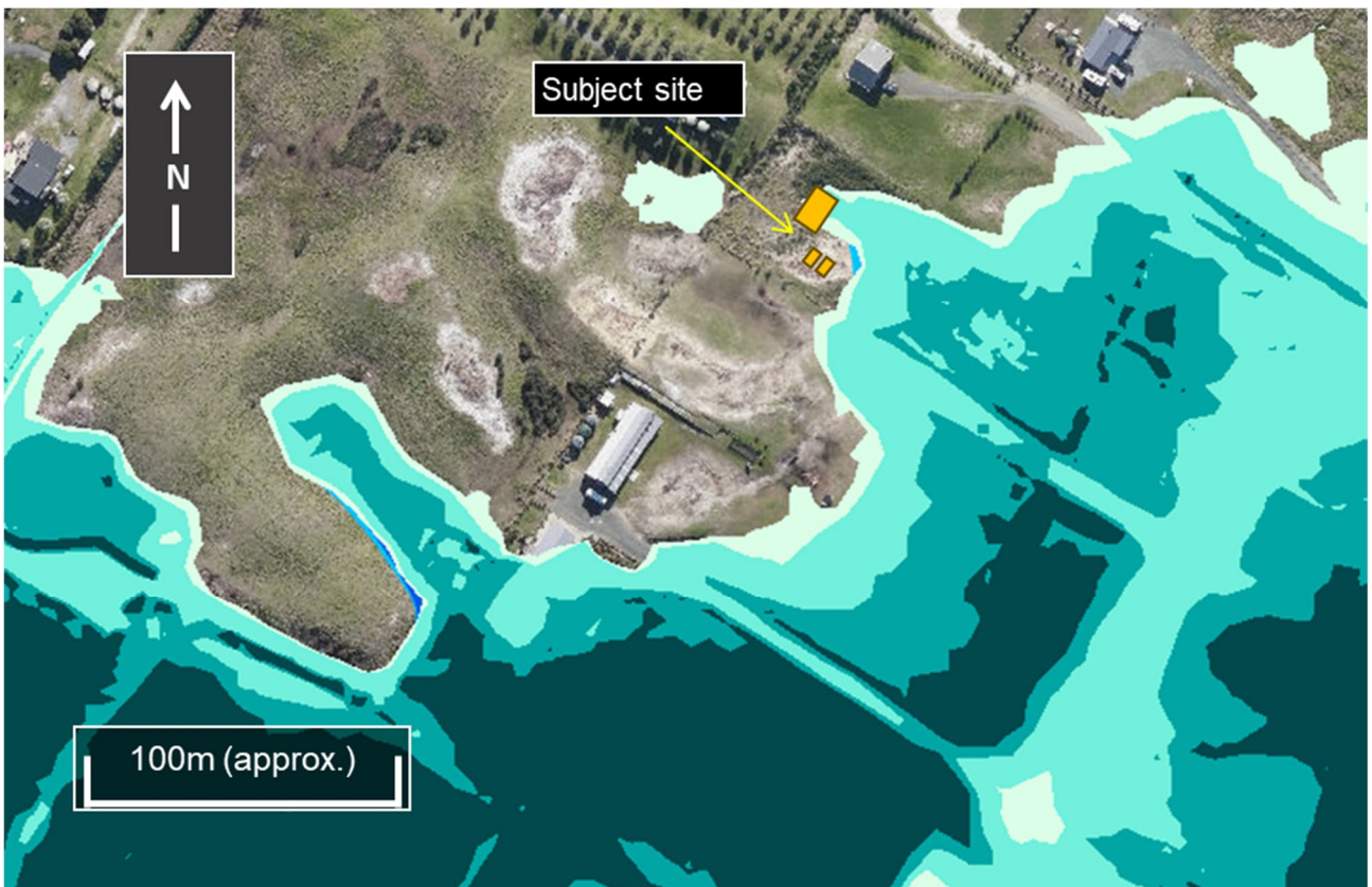
Figure 4 - NRC mapped coastal flood hazard at the site.
