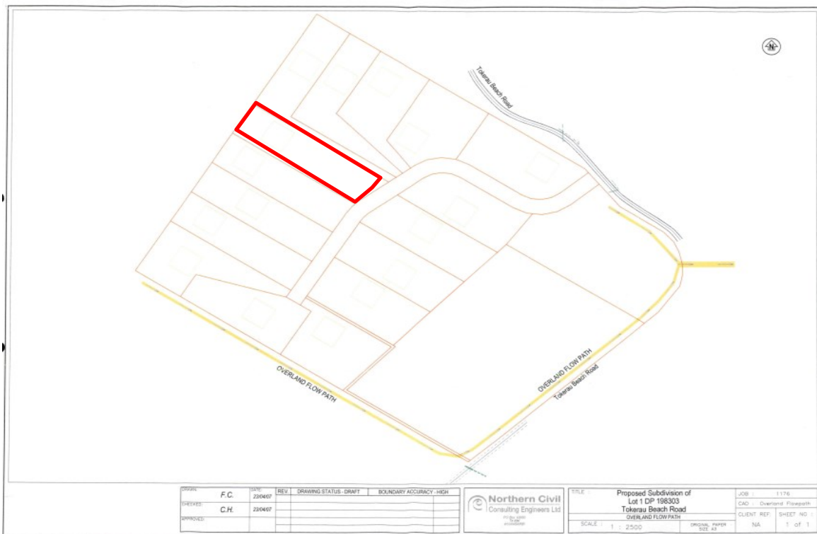
Figure 6: Overland flow path illustrated on the subdivision consent plan (site shown in red line)
