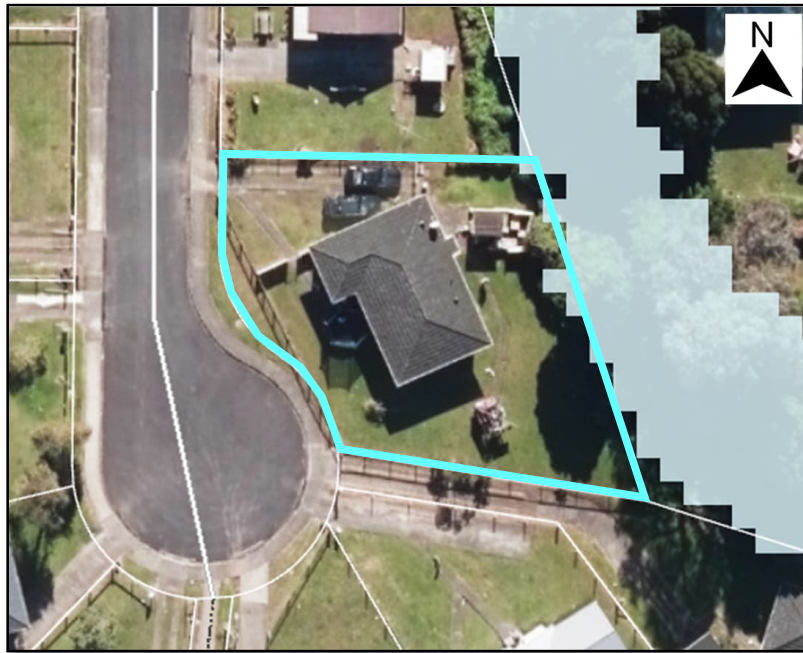
Figure 5: Flood model of the priority river model (light blue colour) for 1% AEP storm with 1% climate change (cyan colour represents site boundary). Source: NRC.
