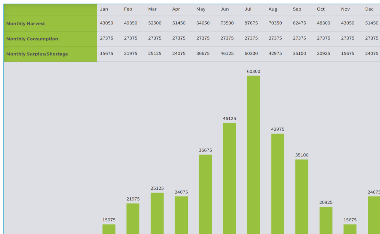
Figure 11: Estimated Potable Rainwater Harvesting Volume from 525m 2 of roof area [Shed and Dwelling] (Source: Devan Tanks)
