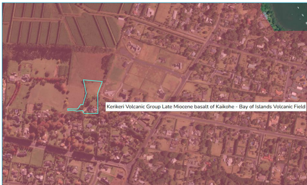
Figure 7: Underlying Geology at the subject site (Source: GNS Maps (Edbrooke & Brook, 2009))
