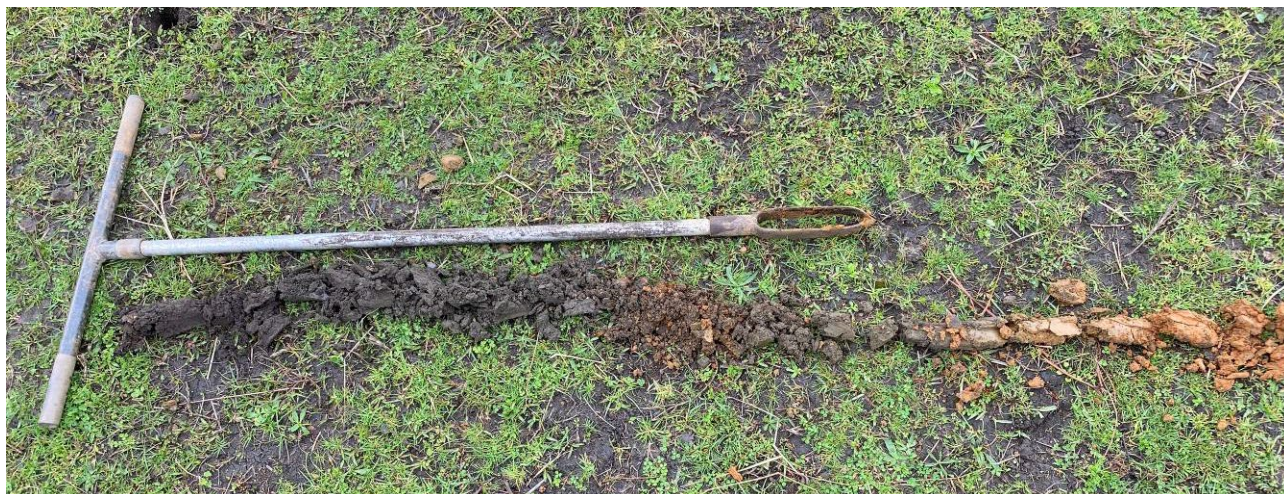
Photograph 2: Borehole showing 400mm of category 5, slightly moist, brown topsoil followed by 100mm of category 4, slightly moist, brown, silty clay loam with gravel. From 500-700mm soils became category 5, slightly moist, brown, silty clay. From 700-1200mm soils were category 6, slightly moist, orange, silty clay.
