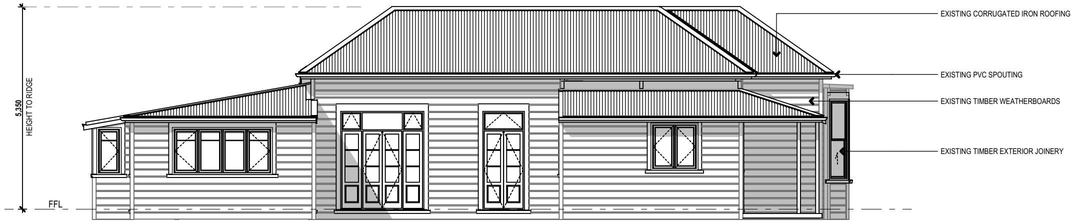
1 A100 EXISTING WEST ELEVATION Scale 1:100
