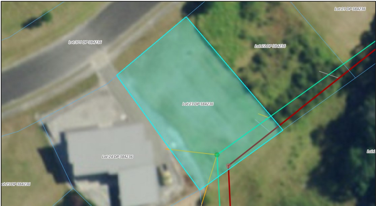
Figure 1: Aerial snip from FNDC Maps showing site boundaries (cyan), public stormwater (green), private stormwater (orange), public wastewater (red) and private wastewater (grey)
