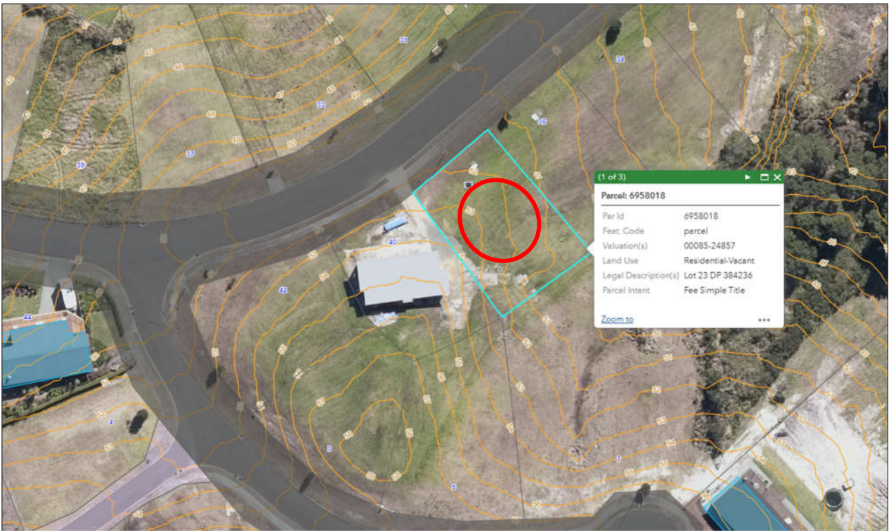
Figure 1: Screenshot aerial view from the FNDC on-line GIS Property and Land Map. 1.0m LiDAR contours are overlaid. Property boundary is highlighted in cyan. Red ring depicts proposed development area.
