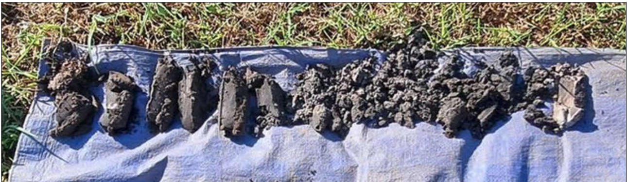
Figure 6: Site photograph of the HA02 soil arisings, typical of the northern and western ends of the development area (0.0m to 1.1m).
