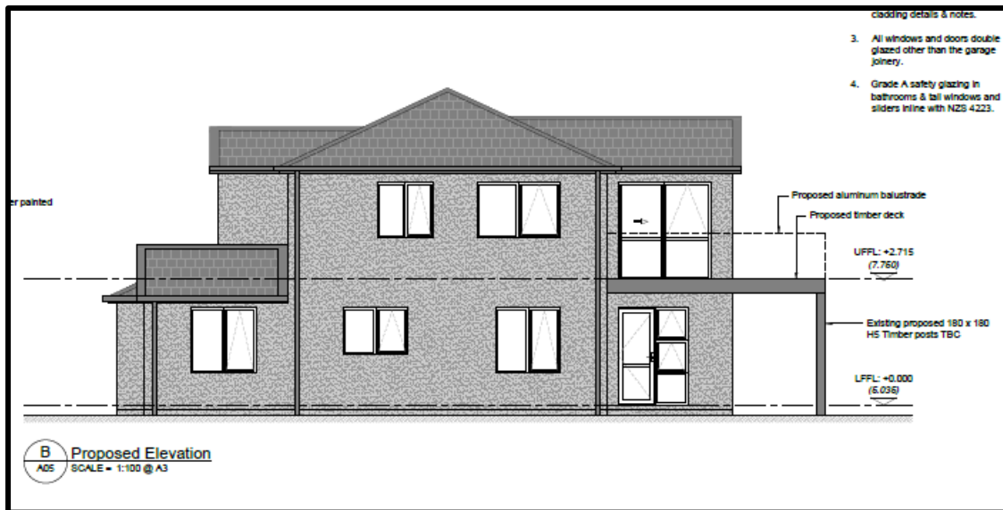
Figure 3: Elevation concept showing upper storey deck.
