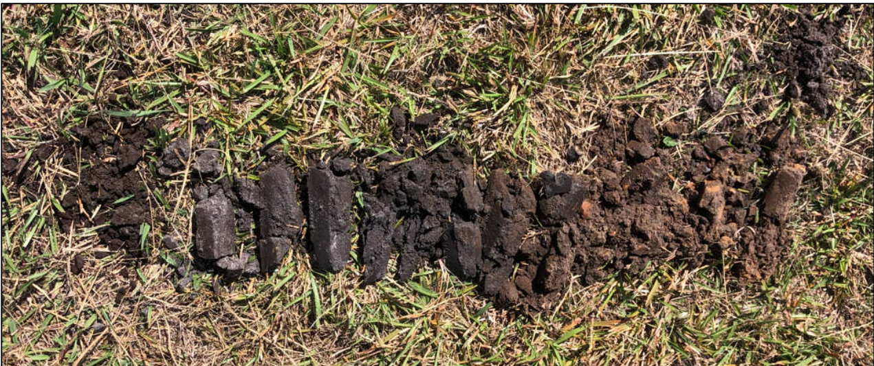
Figure 7: Site photograph of HA01 which were typical of the soil arisings encountered (0.0m to 0.95m).
