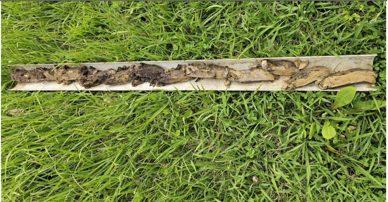
200mm silty loam topsoil over clay loam Class 5, (as per AC TP-58, Table 5.1)
