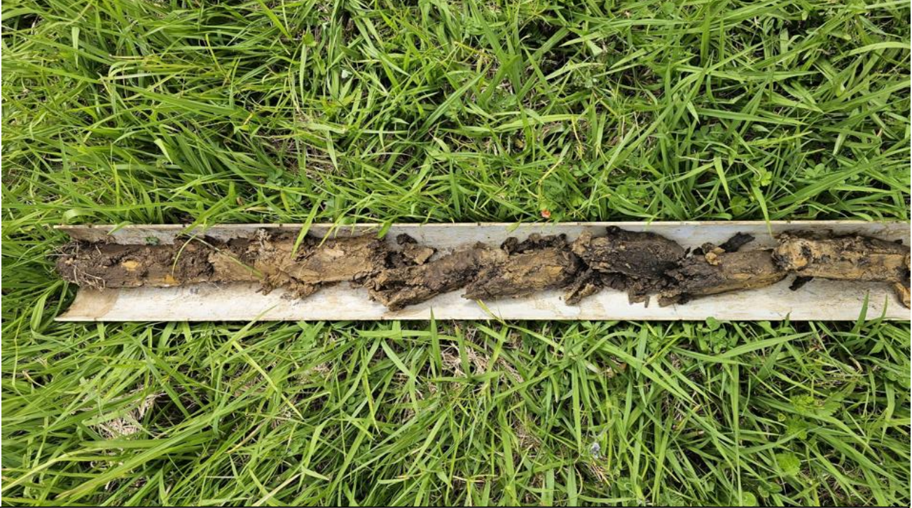
200mm silty loam topsoil over clay loam Class 5, (as per AC TP-58, Table 5.1)
