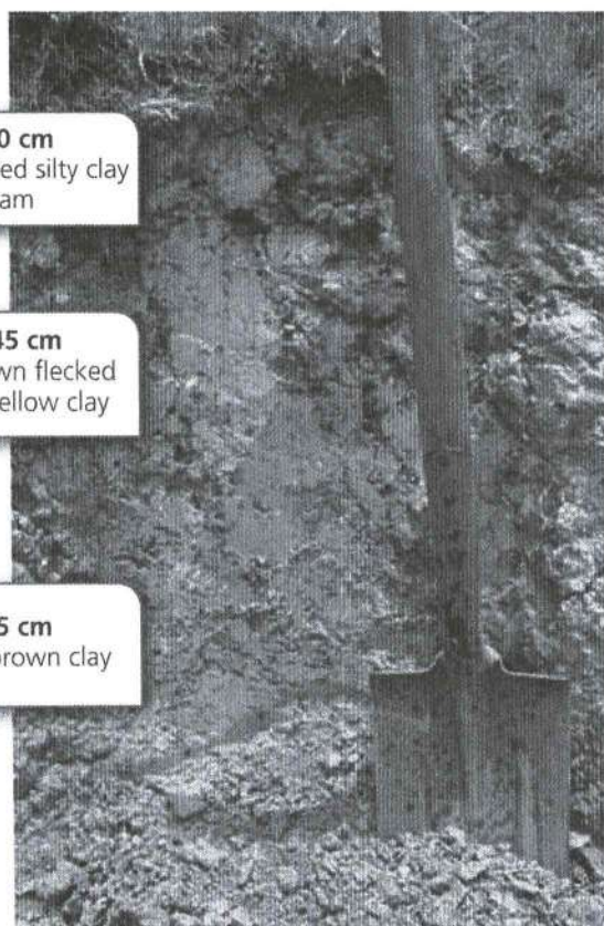
Rangiora clay, clay loam & silty clay loam (RA, RAH) soil profile
