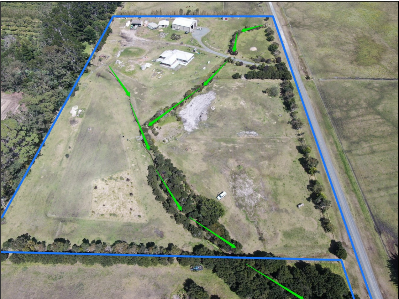
Figure 3: Annotated drone photo of site looking to the southwest, showing parent lot's boundaries (blue) & existing channel (green arrows)
