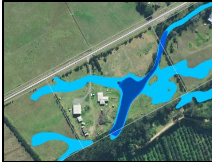
Figure 14: NRC Hazard Maps showing localized flooding around existing drains.
