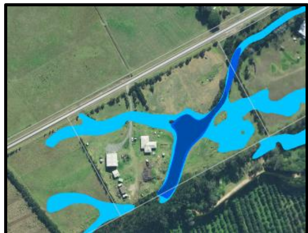
Figure 17: NRC Hazard Maps showing flood susceptibility surrounding existing drains.
