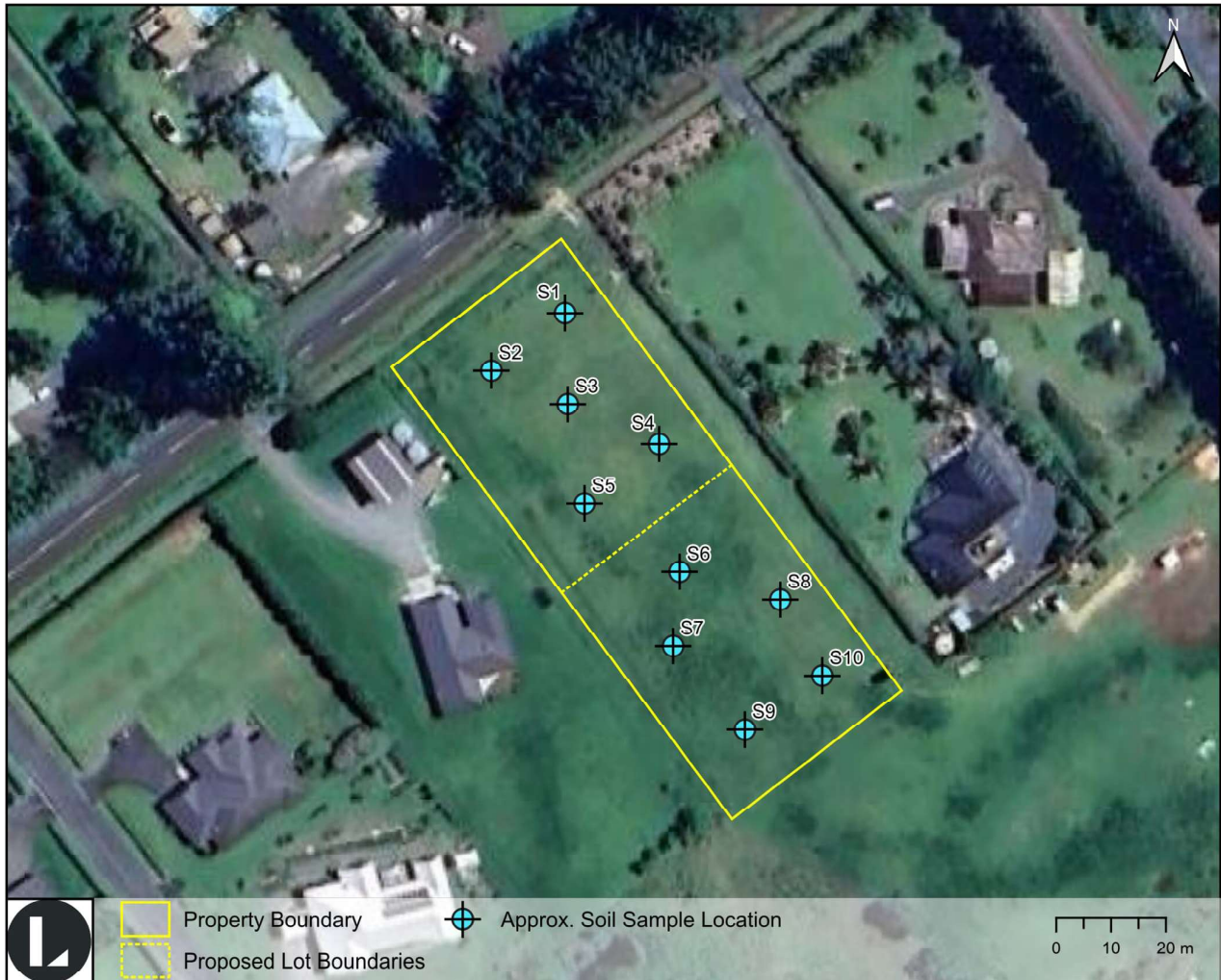
Figure 16. Soil sampling site plan. The approximate soil sampling locations are shown in blue. Source: Google Earth (annotated image).
