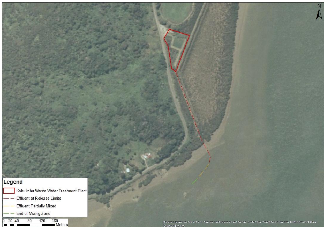
Figure 4: WWTP release points and mixing process
