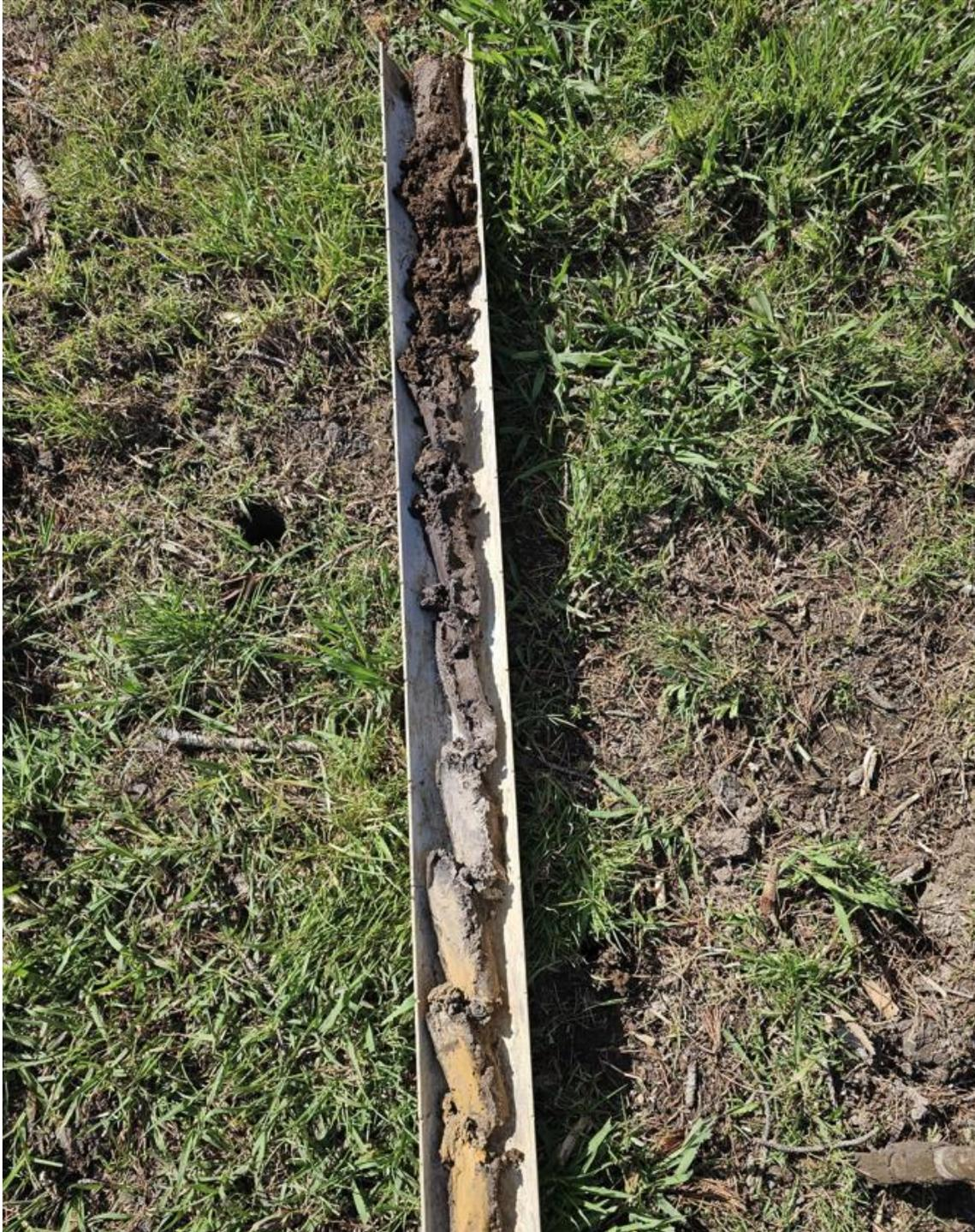
**300mm silty loam topsoil over clay loam
