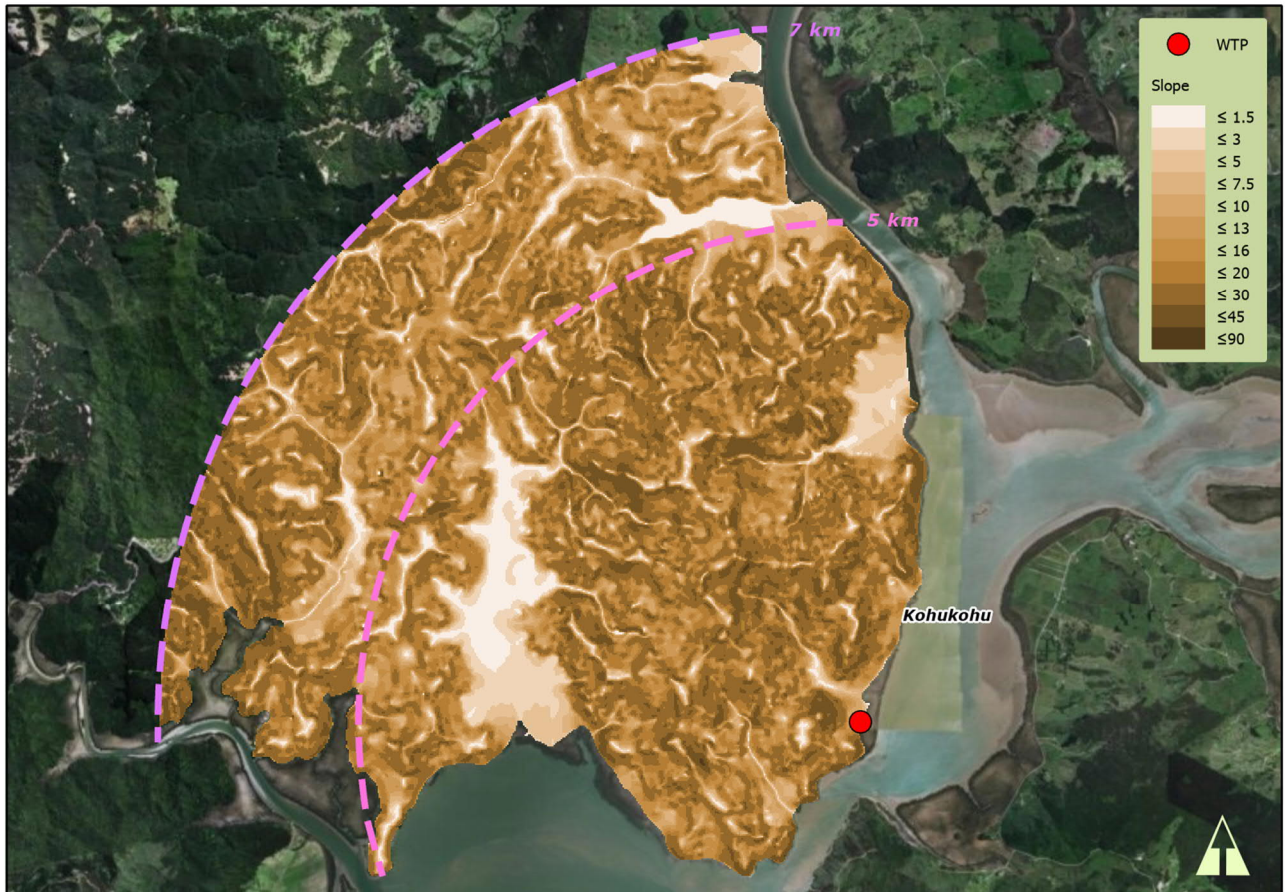
Figure 2-7 Slope levels within a 5 - 7 km radius from the Kohukohu WWTP
