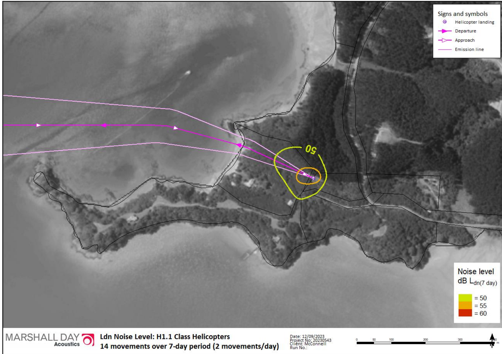
Figure 3: Noise emissions from Helicopter Operation (dB L dn(7 day) noise level over rolling period, 14 x H1.1 helicopter movements)
