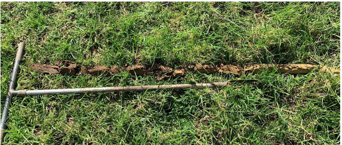
Photograph 1: Showing ~200mm of category 5, slightly moist, brown topsoil followed by category 6, slightly moist, brown, silty clay to a depth of 500mm. From 500-1200mm soils were category 6, slightly moist, orange, silty clay.
