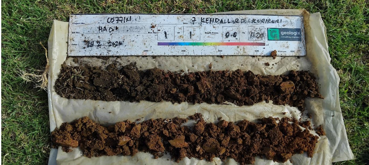
Figure 13: Hand Auger location and soil photo.
