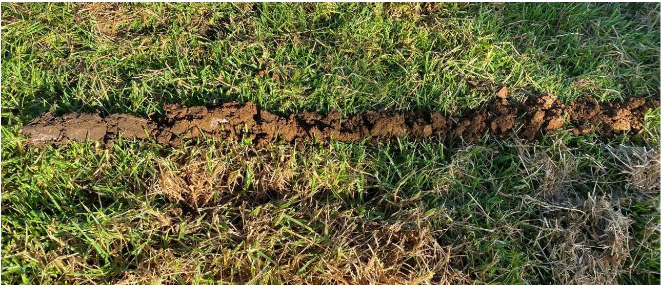
Photograph 2: Borehole showing 200mm of category 4, slightly moist, dark brown, topsoil followed by category 4, slightly moist, brown, friable, silty, clay loam to a depth of approximately 1000mm.
