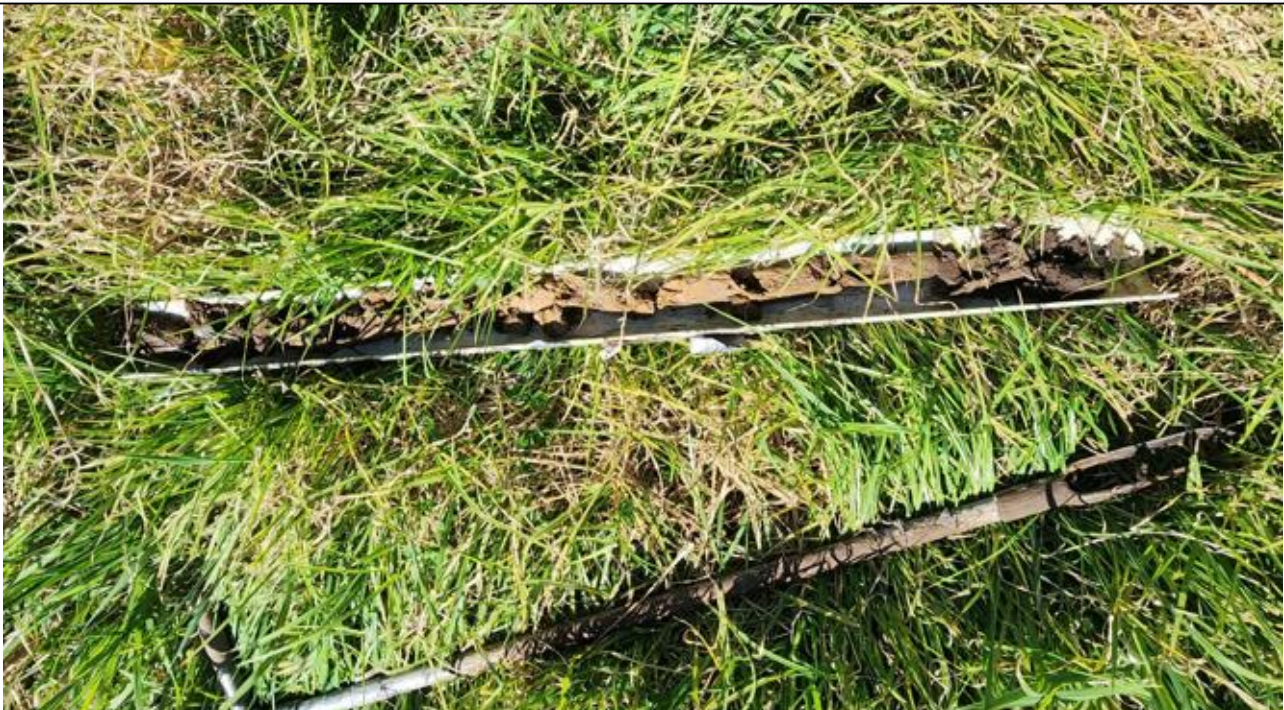
300mm topsoil over silty clay-loam Class 5, (as per AC TP-58, Table 5.1)
