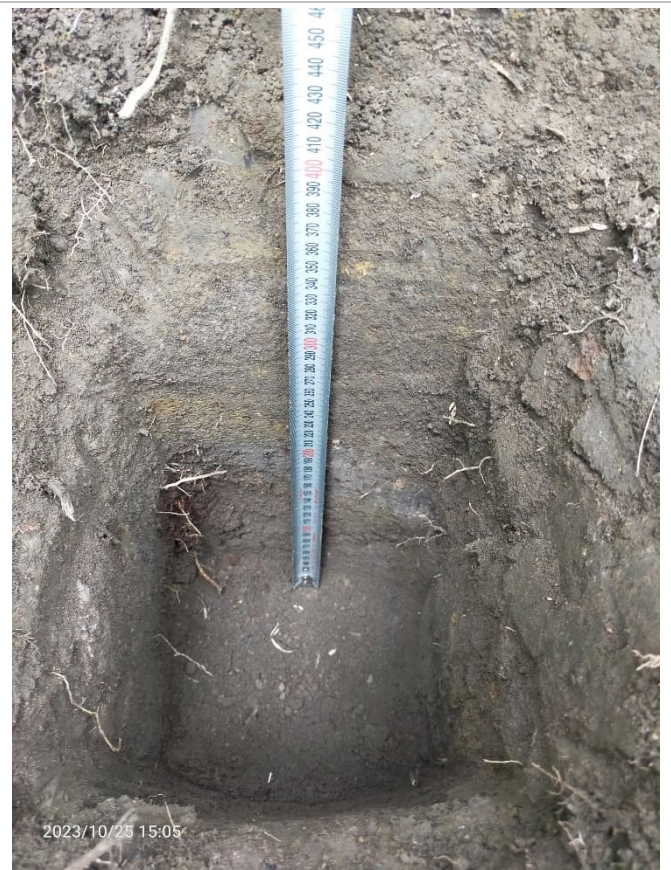
Photograph 8. Typical soil profile encountered within bund.
