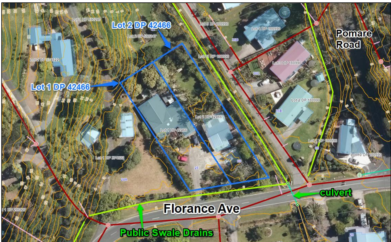
Figure 1: Aerial view of the subject site (blue) with public stormwater (green) and wastewater (red) services and 1.0m contours (orange) from FNDC GIS maps.
