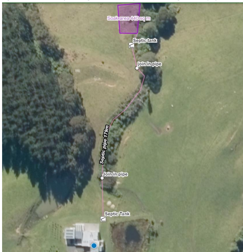
Figure 9: Schematic of Existing Wastewater System (GIS image courtesy of G.Blunden)
