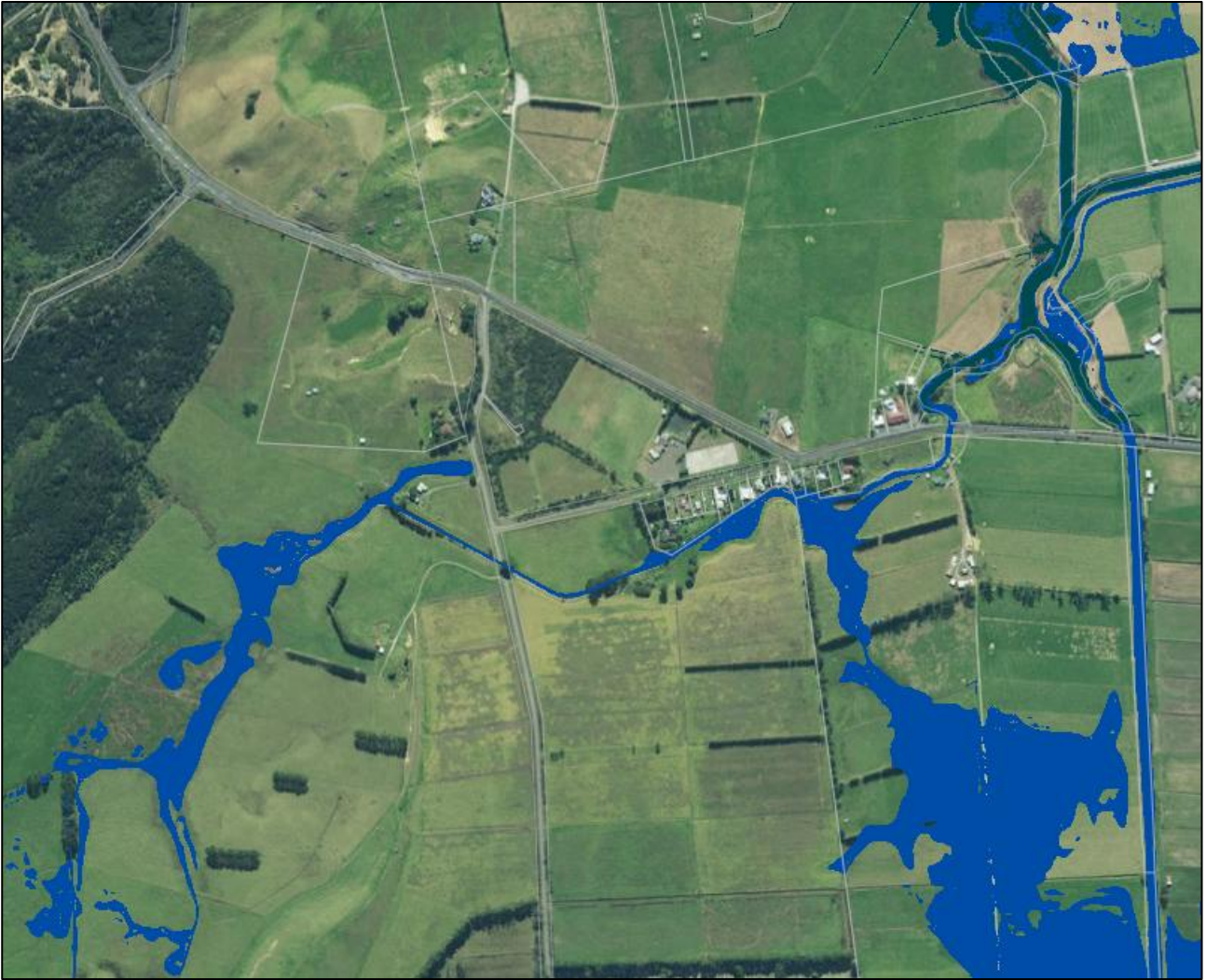
Figure 6 - NRC 10yr. River Flood Hazard Zone (dark blue) for the downstream drainage path. No building affected.
