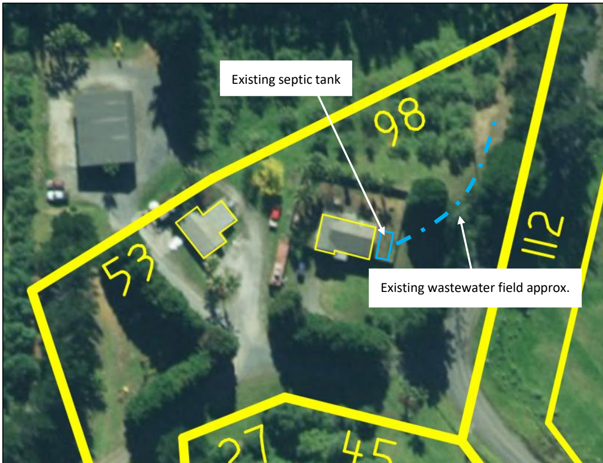
Figure 14 - Lot 5 existing septic tank and wastewater field location (approximate)
