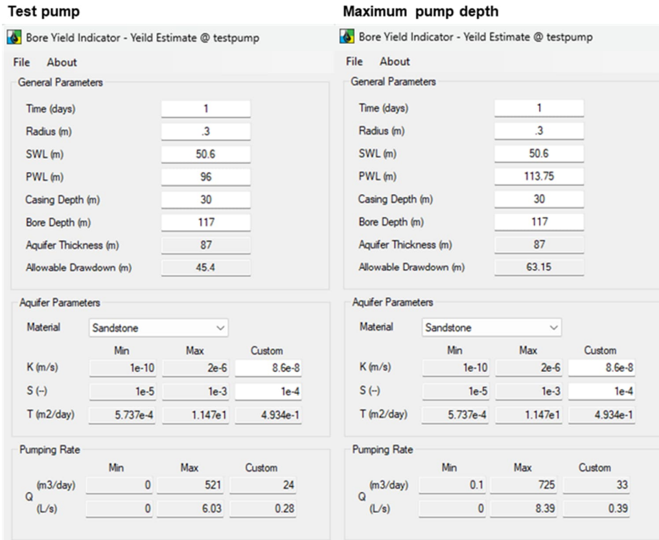
Figure 4. Bore yield indication tool set up for test pumping and maximum pump depth conditions.
