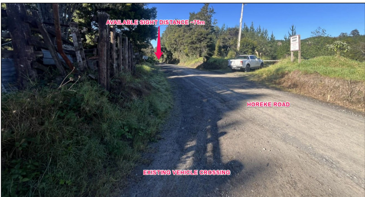
Figure 8: Annotated site photo from vehicle crossing show available sight distance to the south
