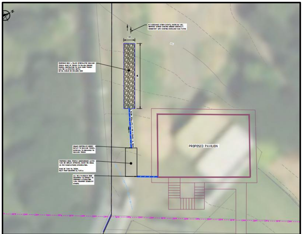
Figure 19: Proposed stormwater management for the pavilion.
