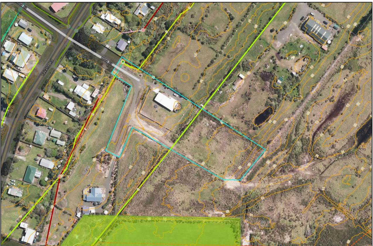
Figure 5: Aerial Snip from FNDC Maps Showing Parent Lot's Boundaries (cyan), 1m contours (orange), Public Stormwater Infrastructure (green) and Public Wastewater Infrastructure (red).
