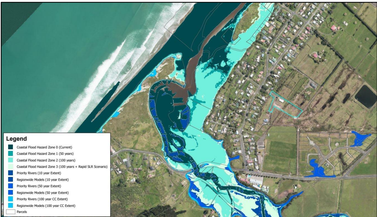
Figure 7: Screenshot from Northland Regional Council (NRC) Online GIS Showing Modelled River & Coastal Flooding Extent.
